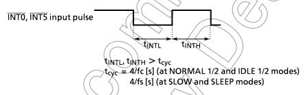
Note 3: If a signal without noise is input to the external interrupt pin in NORMAL 1/2 or IDLE 1/2 mode, the maximum times from input signal edge to input latch set are as described below:
