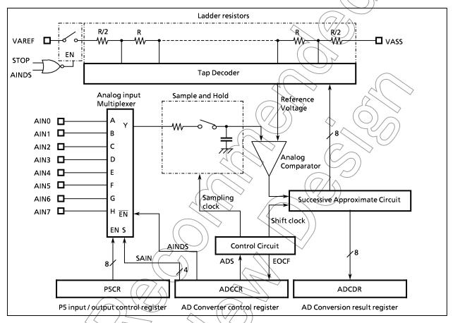
Figure 2-55. AD Converter
