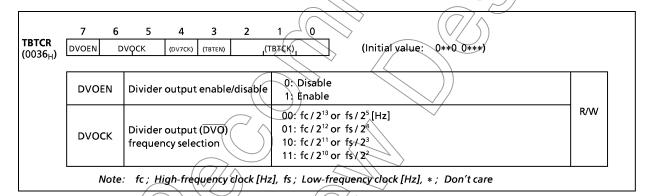
Figure 2-12. Divider Output Control Register
