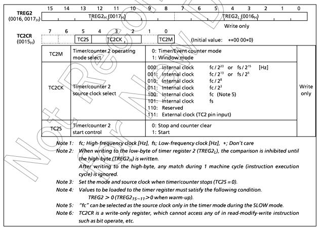
Figure 2-24. Timer Register 2 and TC2 Control Register
