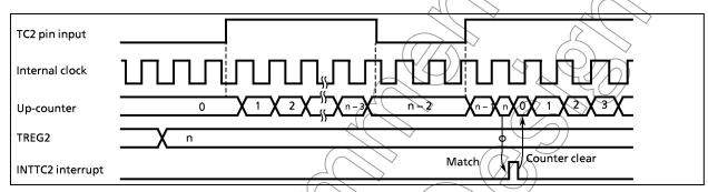
Figure 2-25. Window Mode Timing Chart
