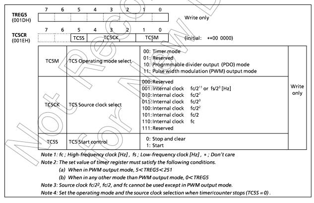
Figure 2-30. Timer/Counter 5 Timer register, Control register
