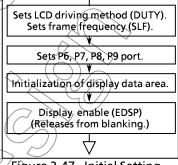
Figure 2-47. Initial Setting of LCD Driver
